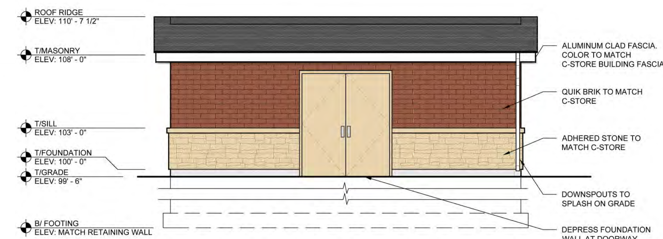
2 COMPRESSOR ROOM NORTH ELEVATION SCALE: 2"
