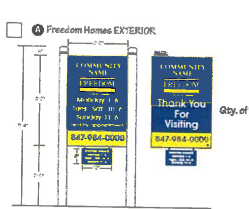
3'-0" x 2'-0" double face mdo plywood sign on wood posts w/ double face hanging hours panel
