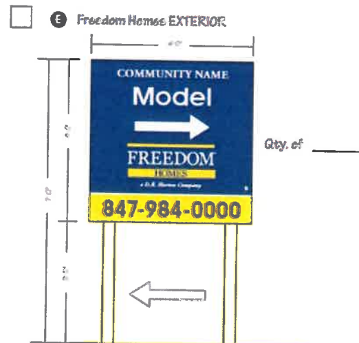
4'-0" x 4'-0" double face mdo plywood sign on wood posts
