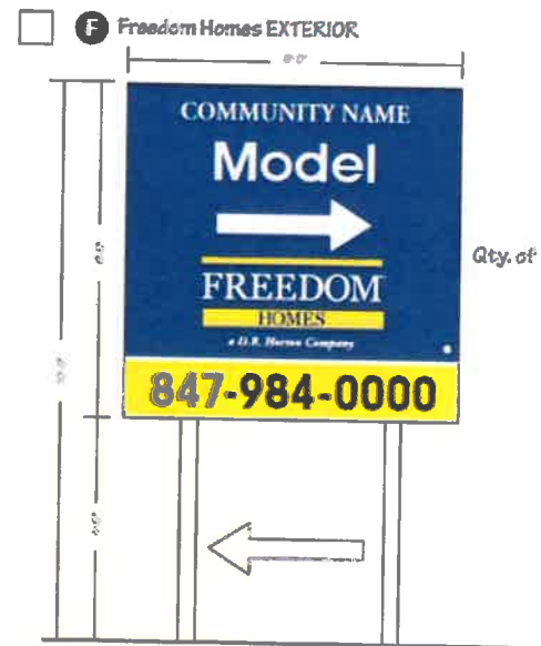
6'-0" x 6'-0" double face mdo plywood sign on wood posts
